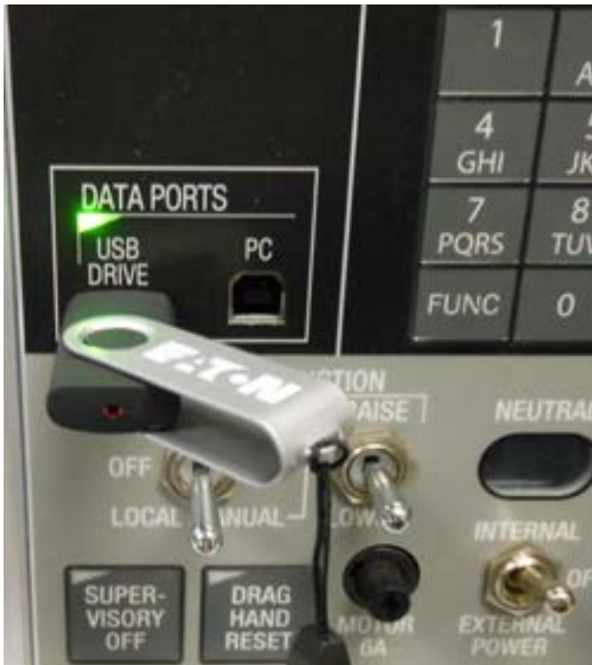
Figure 7-2. A USB memory device in the data port.
