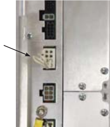
Figure 7-11. DC power jumper in place on side of control. This jumper must be in place to power the control when the substation battery option is not provided.
