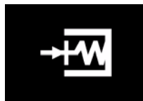
Fig. 25: "Closing spring charged" indication
